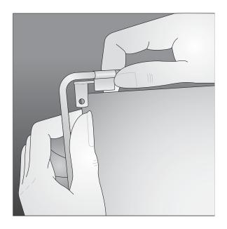
Attach the film carefully to a proper-sized hanger. Attach the lower corners first. Avoid finger marks, scratches or bending.
