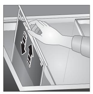
Immediately after immersion in the developer, tap the hanger to dislodge air bubbles. **Agitate for 5 seconds every 30 seconds.**
