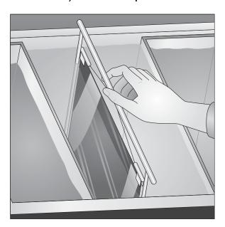
Place the film in the stop bath for **30 seconds**. Then agitate moderately, lift from the stop bath, and drain well.
