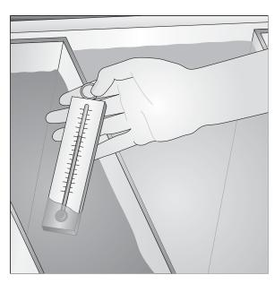
Check the temperature of solutions with an accurate thermometer, rinsing it off after checking each one. Adjust the temperature as needed.
