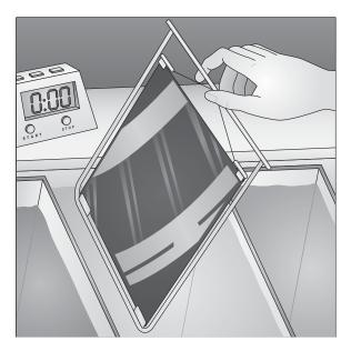
When the timer goes off, quickly lift the hanger out of the developer. Then drain the film **for a moment** into the space between the tanks. For faster drainage, tilt the hanger.
