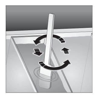
Stir the developer and fixer to equalize their temperatures. Use separate paddles for each to avoid contamination.
