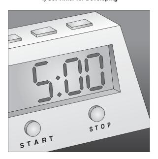
Set a timer. **5 minutes** at 68° F (20° C) is recommended; 4 minutes at 72° F (22° C) if using the KODAK INDUSTREX Film Calculator.
