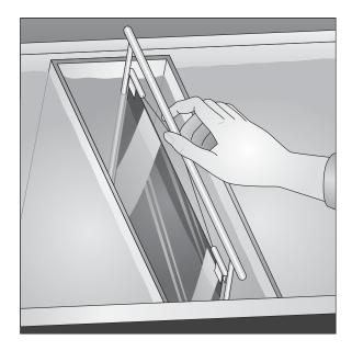
Immerse the film in the fixer for **3** to **6** minutes, agitating for **5** seconds very **30** seconds. Film should remain in fixer for twice the time it takes to "clear" it (when the milky look disappears). Never fix film for less than **3** minutes.
