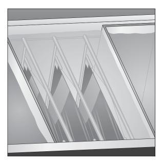
Place the film hangers in a tank of running water for **10 to 30 minutes**. Keep ample space between the hangers (water must flow over the tops).
