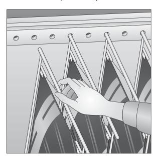
Dry the film at room temperature in a dust-free area or suitable drying cabinet. The temperature must not exceed 120° F (49° C). When the film is dry, remove from hangers and insert into envelopes.
