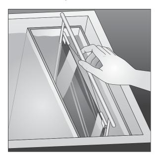
If facilities permit, use a final rinse of KODAK PHOTO-FLO Solution to speed drying and prevent water marks. Immerse film for about **30 seconds**, and then drain for several seconds.
